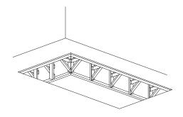
2. **Recessed Installation:** Suggested stud construction is illustrated.
